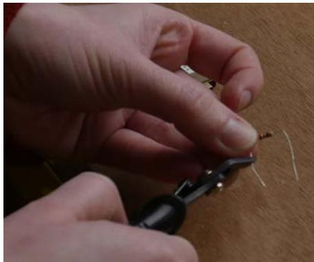
Put the components in the right place on the electronic board. Make sure you use the right resistor with the right leg!
