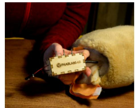
Make three holes in the back of the bear and put the switches through those holes. Secure the switches with nuts to the fur of the bear.
