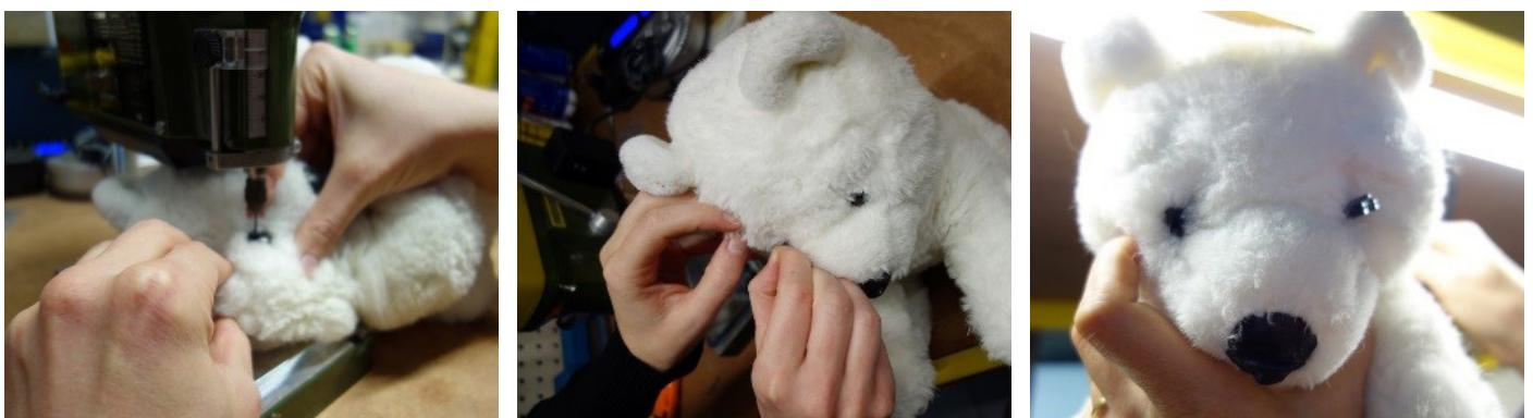
Pull the optical fibre through the drilled hole to the opening of the bear. Attach the optical fibre with superglue to the plastic eye. Make sure the optical fibre cannot move anymore while working on the bear.
