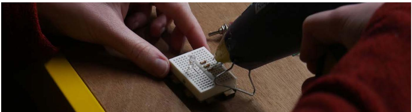
Connect the black wire of the battery conenctions to the GND (ground) leg of the white LED. Secure this connection on the electric board also with hot glue.
